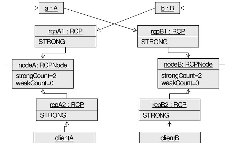
**Figure 6.** Simple circular reference between two objects.
