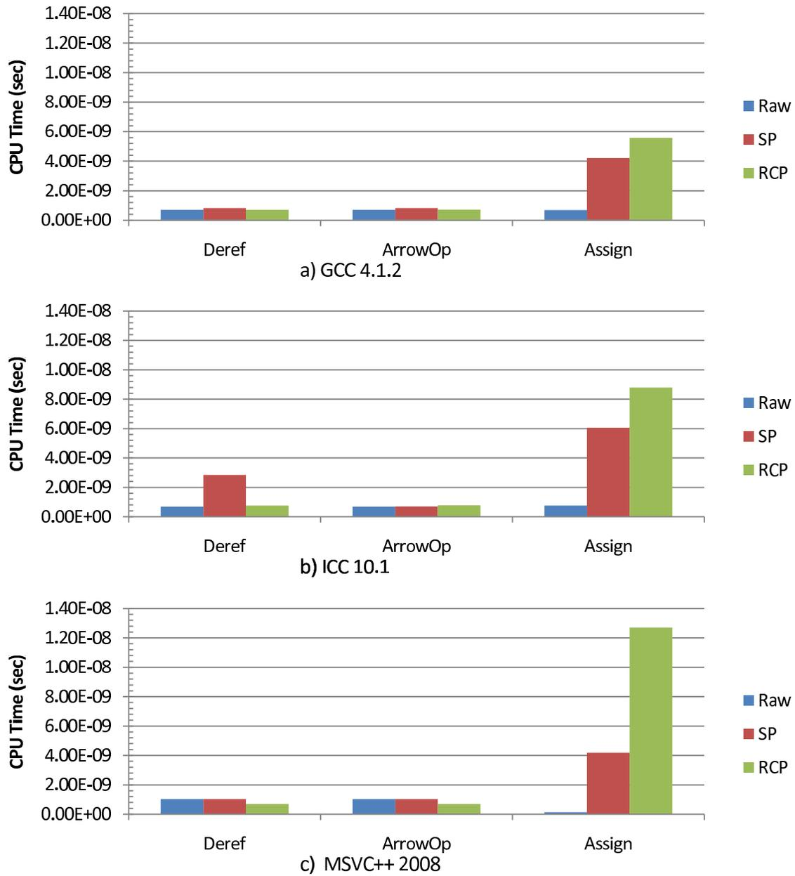
**Figure 13.** Timings of basic RCP operations on for three compilers
