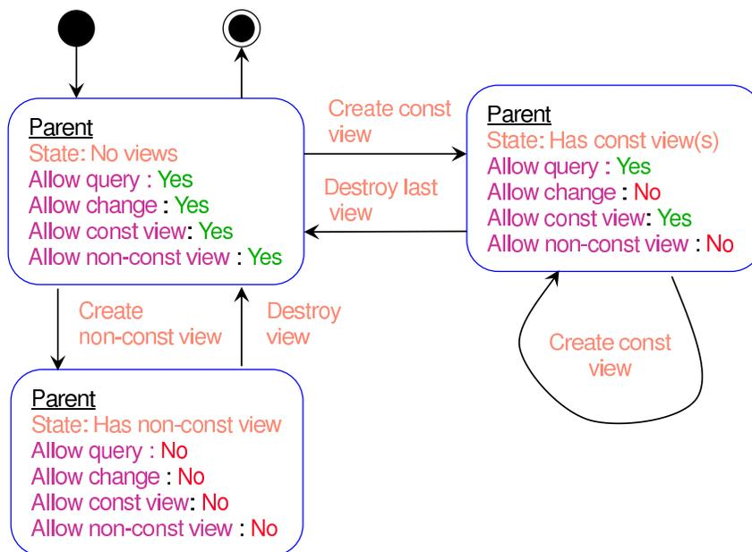
**Figure 17.** State behavior for parent object in “generalized view” design pattern.
